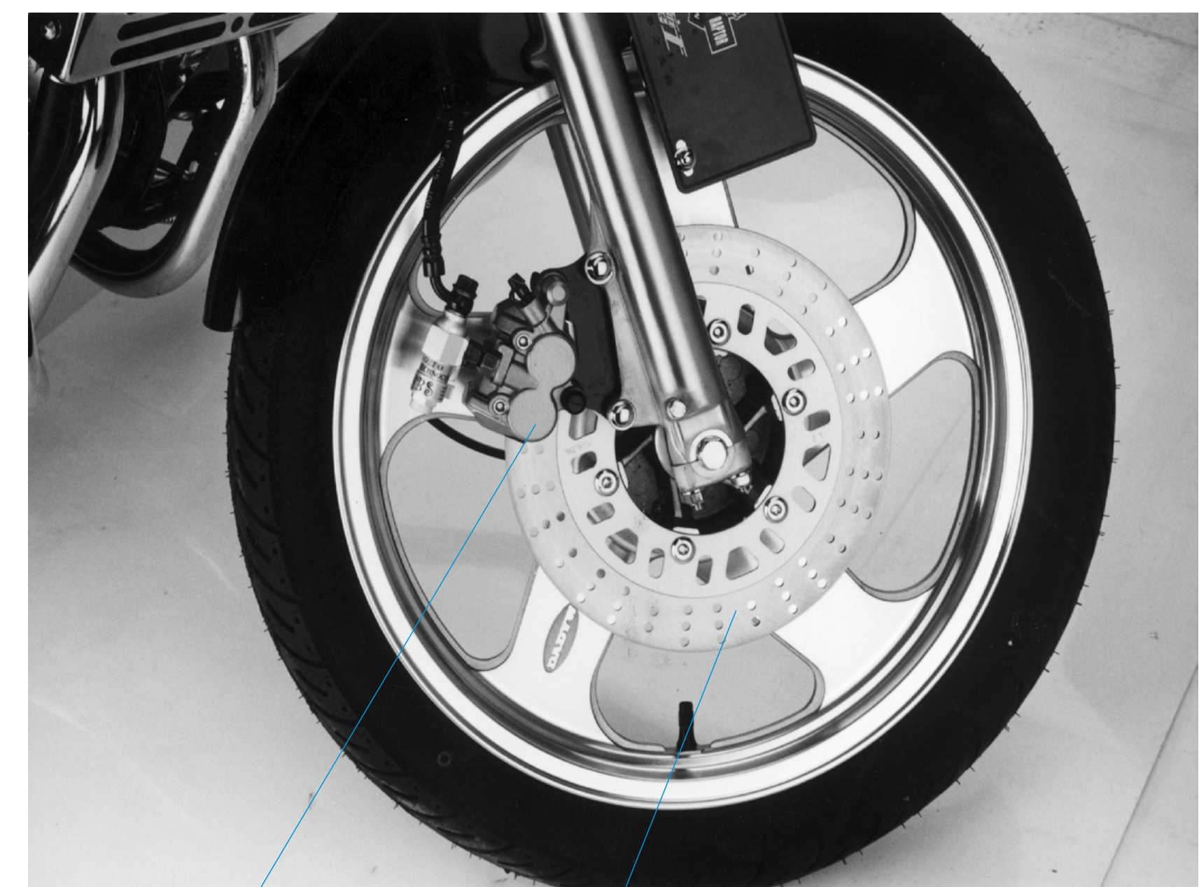
Brake calipers Brake disc
