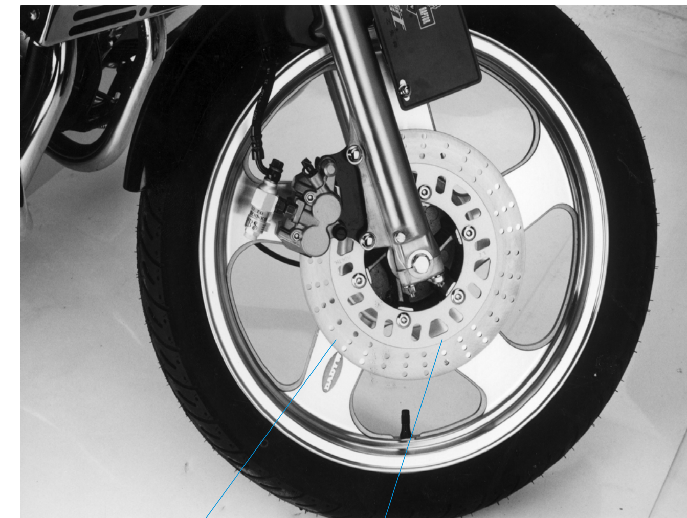
Brake disc Wear mark
