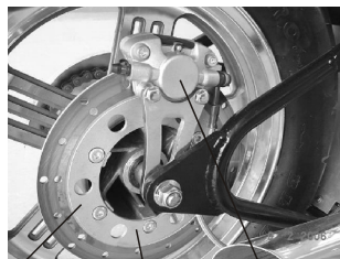
wear mark brake disc brake calipers
